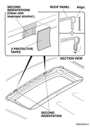
7. Remove the adhesive backing from the two protective tapes, and attach one to the roof panel at each second indentation.
