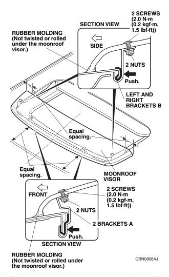
13. Tighten two screws and two nuts on the front of the vehicle first, then tighten two screws and two nuts on each side. Tighten while applying pressure so that there is no gap between the roof panel and the brackets A and B. Torque the screws to 2.0 N·m (0.2 kgf·m, 1.5 lbf·ft).
